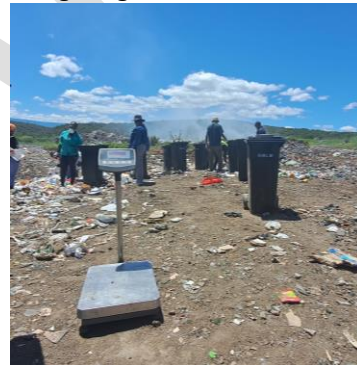
Figure 4-10: Scale used for weighing of waste
